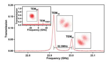
FIG. 3. (Color online) Cavity transmission vs the scanning of the probe frequency. The inset shows the  $\text{TEM}_{00}$ ,  $\text{TEM}_{10}$ , and  $\text{TEM}_{01}$  modes. Splitting ~82.5 MHz between  $\text{TEM}_{10}$  and  $\text{TEM}_{01}$  mode is observed. Three images, from the left-hand side to the right-hand side, are the 2D intensity distributions of  $\text{TEM}_{00}$ ,  $\text{TEM}_{10}$ , and  $\text{TEM}_{01}$  modes directly detected by a CCD camera, respectively.
